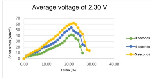
Figure 9. Result of peel test 2.30 V
