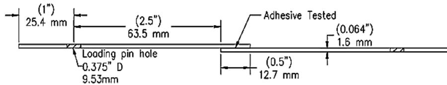
Figure 2. Standard of shear test of ASTM D1002
