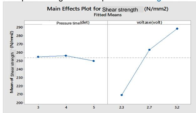
Figure 12. Main Effects Plot of shear strength
