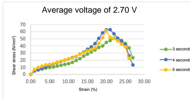
Figure 10. Result of peel test 2.70 V
