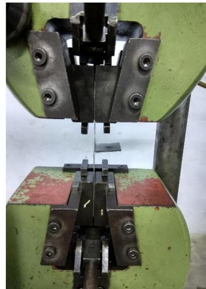
Figure 5. The peel test
