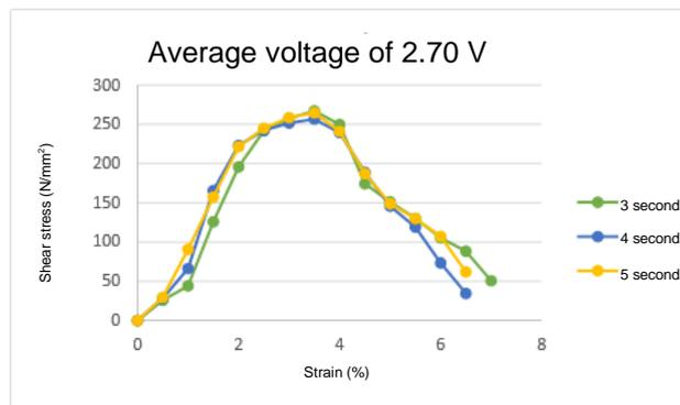
Figure 7. Result of shear test 2.70V
