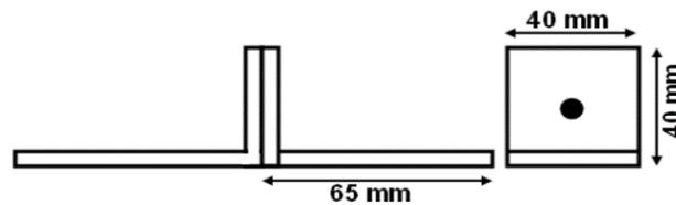
Figure 3. Standard of Peel Test of ASTM D1002
